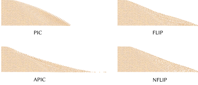
Fig. 5. The collapse of a sand column. When initialized on vertical lines, the sand particles could stay in the same (but curved) line due to the positional trap during the collapse when simulated with PIC, FLIP, or APIC. Advecting with NFLIP, on the other hand, would eliminate this artifact.
