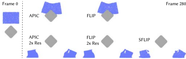
Fig. 11. Fracture. A rectangle with the NACC plastic model falls onto a wedge and then collides onto the ground. The rectangle breaks into pieces with SFLIP, FLIP (2× resolution) and APIC (2× resolution).
