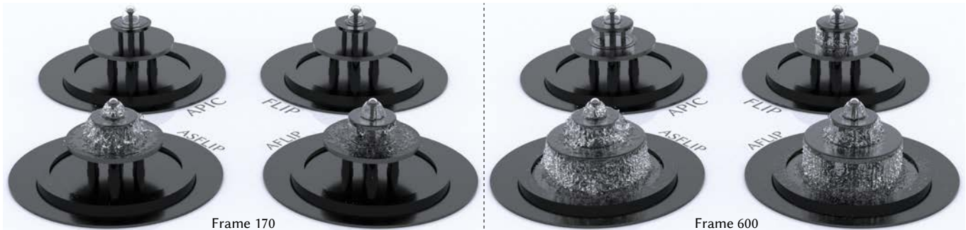
Fig. 1. Water Spray from a Fountain Nozzle. Weakly-compressible water is simulated with the material point method. A weak frictional coefficient (0.0125) is applied between the liquid and plates. AFLIP and ASFLIP induce much less dissipation than the traditional methods, so liquid particles are more spread out within the same period. Particles advected by ASFLIP are also more energetic than AFLIP when leaving the top plate since particles are used to assist friction computation. ©2021 Tencent
