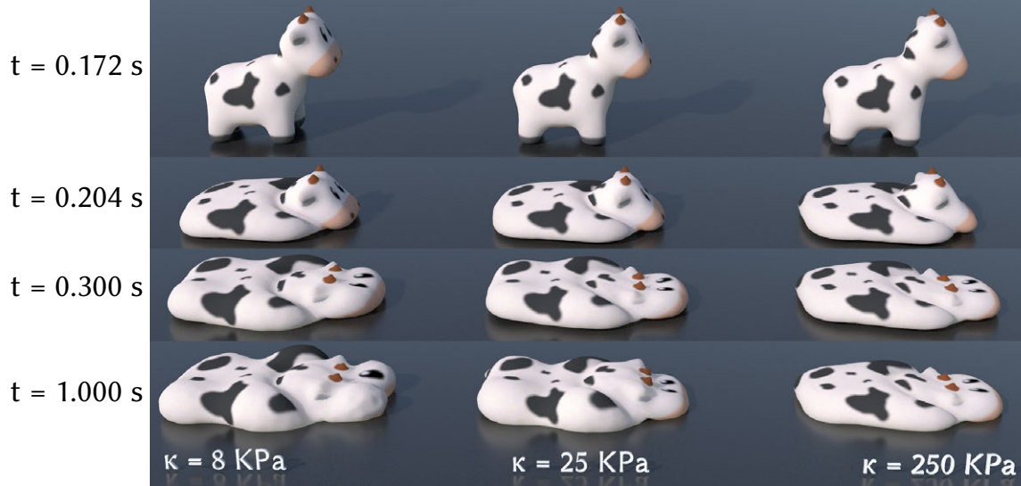
Figure 13.7: Simulated cream with a wide range of bulk moduli ( \kappa ). Cream with a lower bulk modulus \kappa shrinks or dilates more easily during the simulation, and has a larger volume in the steady state.
